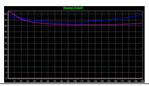
As the Compare function can show only 2 swept graphs at the most, if Compare is activated and a third sweep test is conducted, then the swept graph of the first sweep test will be replaced by the third sweep test. If a fourth sweep test is conducted, then the swept graph of the 2nd sweep test will be replaced by the fourth sweep test and so on. The two graphs in the Compare mode are displayed in a FIFO (first-in-first-out) manner.
