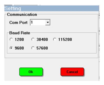
3. Click on the OK button. The PC software and the LCR-6000 will try to establish a connection (success), or an error message appears (fail). If the connection is successful, the windows header (title bar) for LCR-6000 PC software will display the comport and baud rate of the connection.
