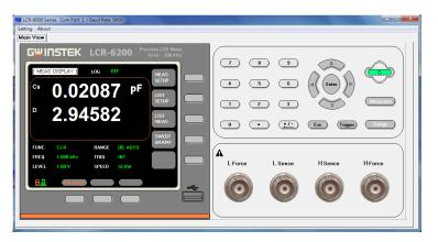
6. After the software and meter have synchronized, the measurement readings and settings from the meter will be displayed on the software display. For future reference, we will call these readings "synchronized parameters".
