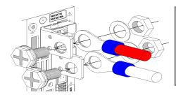
Attach a round crimp-style terminal (inner diameter of at least 6.4 mm) to the load cable.
