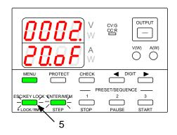
This setting must be specified while the output is off.
