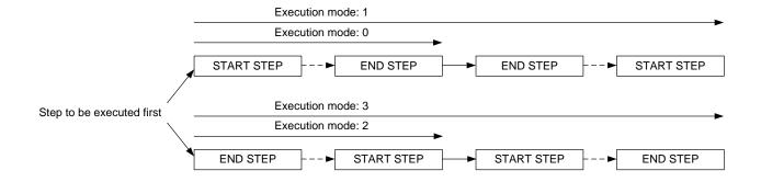
Automatic execution cannot start from a step that is in the middle of the sequence program.
