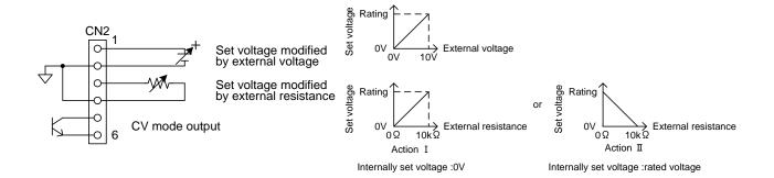
Set voltage control via external signa (Valid when pin No.4 of SW1 is on)
