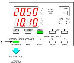
While key lock is activated, the output can be turned off. However, if the output is already off, it cannot be turned on.
