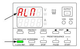
If the voltage and current indicators display "AC oFF" and then "AL $\Pi$ ", and the power switch has not been turned off, there may be a unit malfunction. Perform the following steps:
