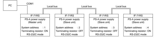
Slave units are designated by using the ADRS command to specify the system address numbers. Slave units in which IF-70GU boards have been installed can be used.
