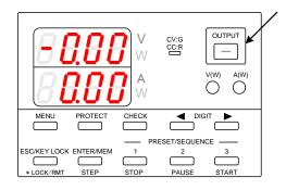
In the PS-A power supply unit, when the output of the unit has been turned on through the external contacts of the analog IF board, the OUTPUT key on the front panel can be used to turn the output on or off during operation. Thus, in case of an emergency where the power supply from the unit to the loads must be stopped, the power supply from the unit can be stopped without needing to turn off the power switch.
