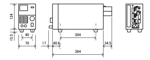
• 800W model : Outside dimensions: 124mm (H) × 140mm (W) × 364mm (D) Weight: Approx. 5.3kg
