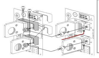
Remove the M3 screws (4 screws) from the positive and negative rear output terminals and the positive and negative voltage remote sensing terminals, and then remove the positive and negative shorting bars.
