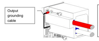
Run the load cable and the voltage remote sensing cable through the output terminal cover, and then fix the output terminal cover to the unit, using the two large screws with washers.
