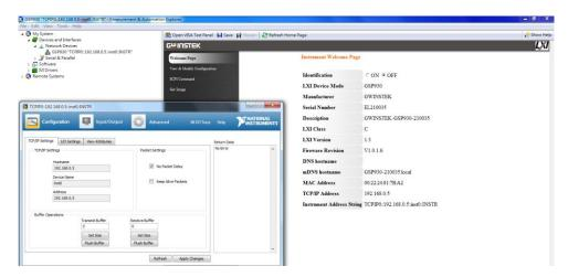
To check that data can be read from the spectrum analyzer, you can go to the NI 488.2 Input/Output setting and execute the \*IDN?\n command.
