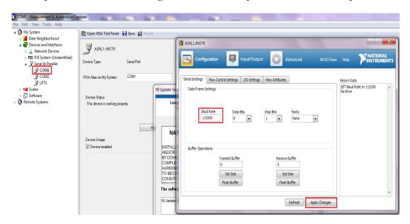
To check that data can be read from the spectrum analyzer, you can go to the NI 488.2 Input/Output setting and execute the \*IDN?\n command.
