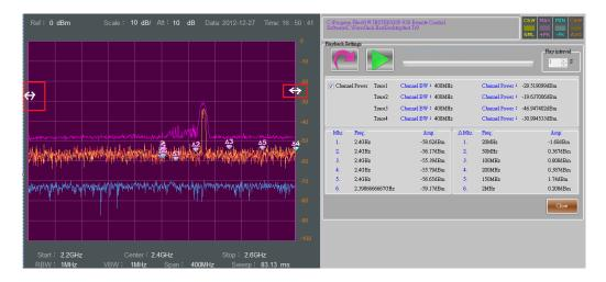
For example, below the 'Channel BW' was set to '40MHz' to measure the 'Channel Power' of 'Trace 1~4'.
