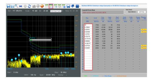
You can tick the 'Open Interval' check box in the Peak Search panel. A purple-colored background will be displayed on the screen to indicate the bandwidth.
