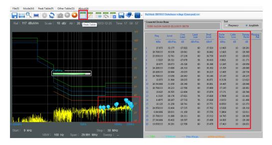
When some frequency points exceed the Fail/Warning Mask, "Warning" or "Fail" will be displayed on the screen.
