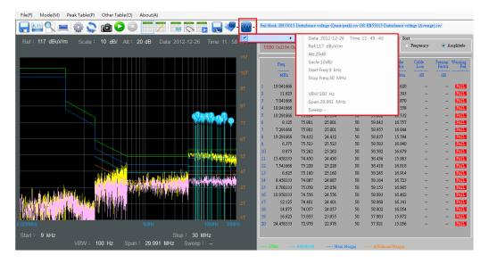
If you want to store the test result of a DUT in a text file, you can press the 'Save to rtf' button. The tables will then be saved in the rich text file format (\*.rtf). An informative description of DUT can be entered and saved under the "Title" tab.
