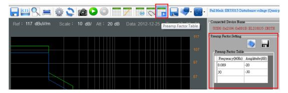
The Probe, cable loss and Pre-amp settings are saved in a \*.csv format, which can be opened and edited by Microsoft Excel.
