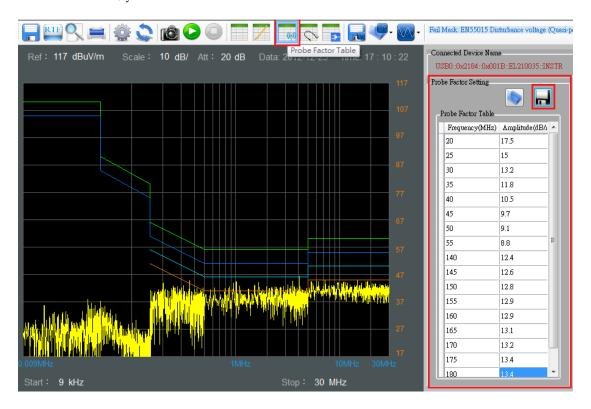
If you know the insertion loss of the cable, LISN, or pulse limiter, it can be inserted and stored in this column.
