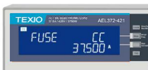
Turbo : OFF, Fuse mode Test result screen
