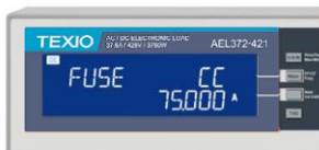
Turbo ON, Fuse mode Test result screen
