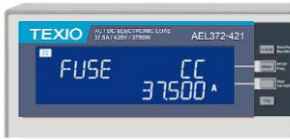
Turbo : OFF, Fuse mode Test result screen
