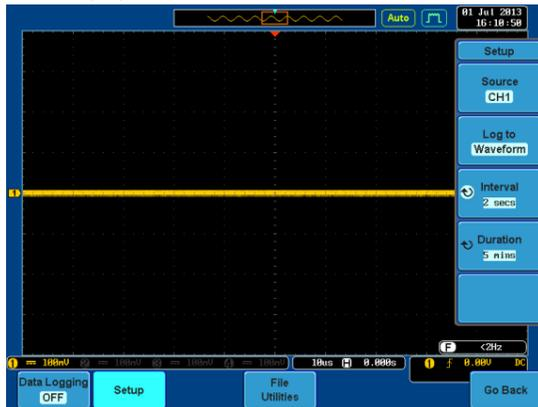
4. Press the *Source* button from the side menu to select which channel to record.
