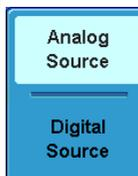
4. Digital Source is enabled when installing the logic analyzer option.
