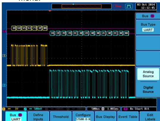
3. Select the Source Input from the side menu. Analog Source:CH1 – 4
