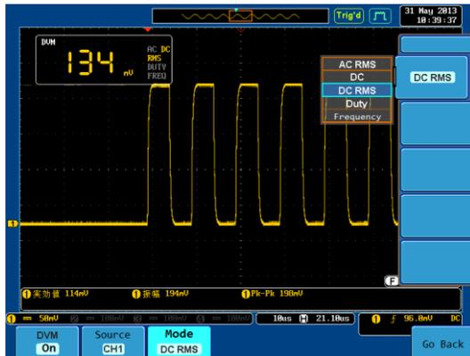
3. Press the Source key to select the input source.(CH1,CH2,CH3,CH4)
