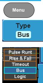
4. Press the Trigger On button from the lower menu and then select the desired Trigger ON condition using the Variable knob and Select key.
