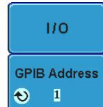
4. Use the Variable knob to set the GPIB Address from the side menu. This option will only be available when the GPIB module is installed.
