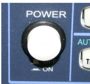
Before using the DL-1060 DMM, taking off the black rubber ring from the Power Switch
