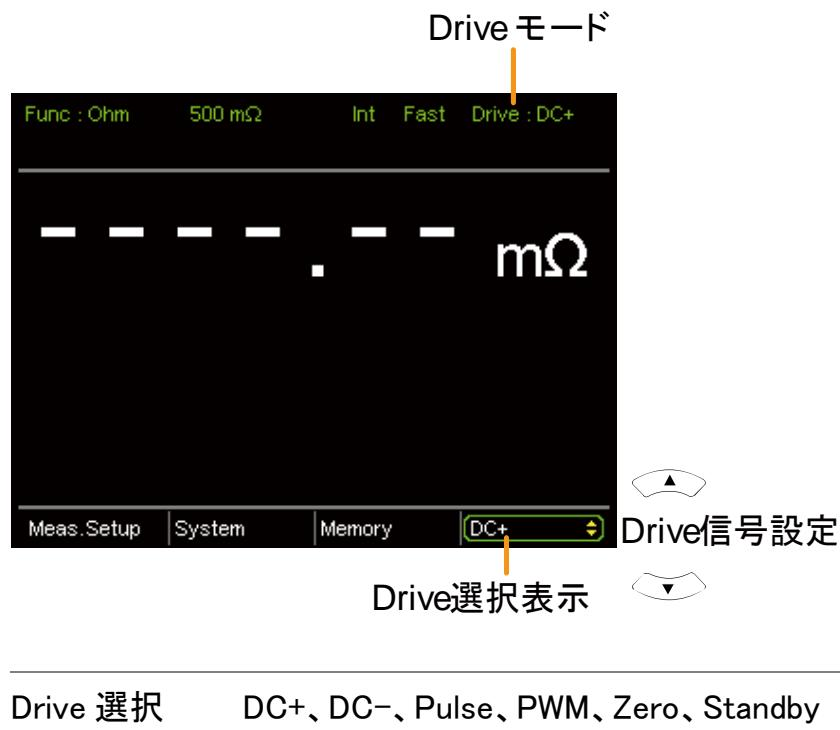
Drive 選択 DC+, DC-, Pulse, PWM, Zero, Standby
