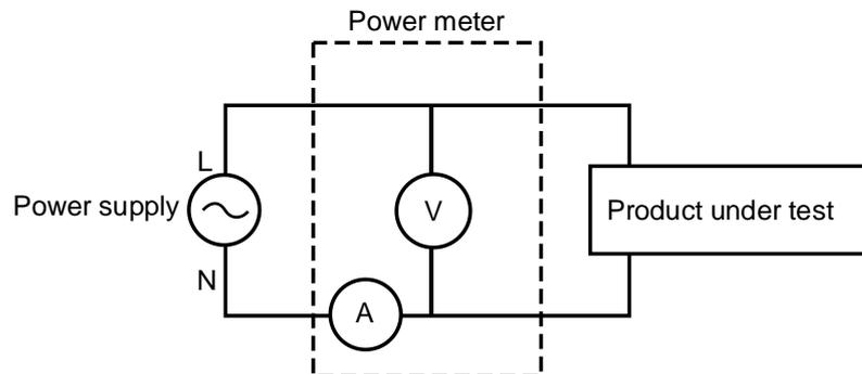
$$\text{機器損失} = (\text{入力電圧 [V]})^2 / 2\text{M}\Omega$$
