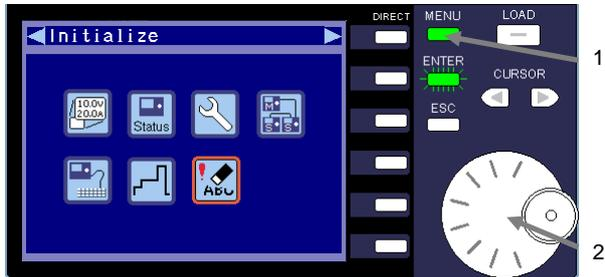
1 Press the MENU key while the unit is in LOAD OFF mode to display the menu window.
