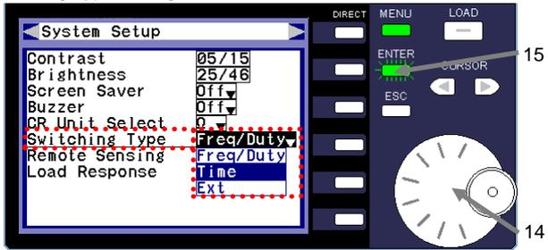
14 Specify the switching type used by the switching function.
