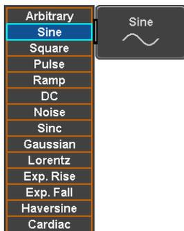
**選択波形** Arbitrary, sine, square, pulse, ramp, DC, Noise, Sinc, Gaussian, Lorentz, Exp. Rise, Exp. Fall, Haversine, Cardiac.
