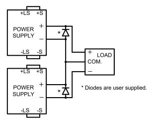
Fig.4-3: Series connection for positive/negative output voltages
