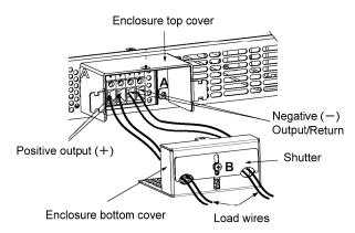
Fig.2-7: Mounting for Output protect cover
