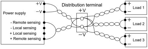
Fig.2-12: Multiple loads connection with distribution terminal
