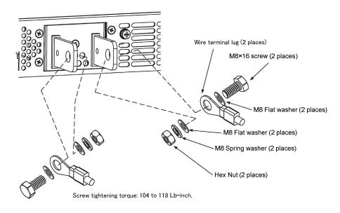
Fig. 2-4: Load wires connection, 6V to 60V models.
