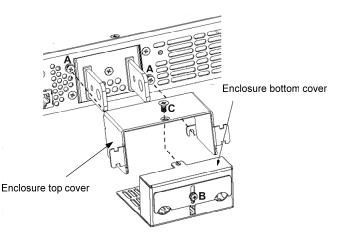
Fix the bus-bars enclosure top cover using the screws marked "A". Loosen screw "B" to release the shutter. Insert load wires through enclosure bottom cover opening and connect load wires. Assenble the enclosure bottom cover by using scre "C". Tighten screws "B" after sliding down the shutter.
