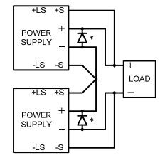
Fig.4-1: Series connection, local sensing
