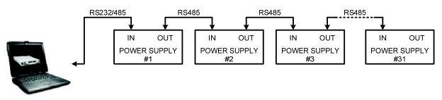
Fig.6-5: Multi power supplies RS232/485 connection
