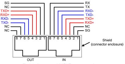
Fig.6-1: J3 rear panel IN/OUT connectors pinout
