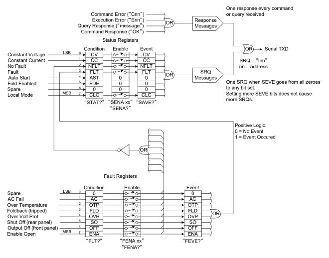
Fig.6-7: Status and Error Registers Diagram
