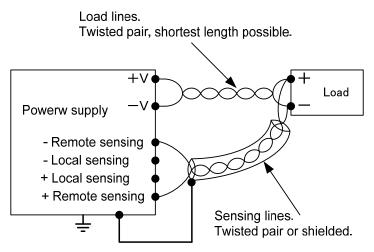
Fig.2-10: Remote sensing, single load
