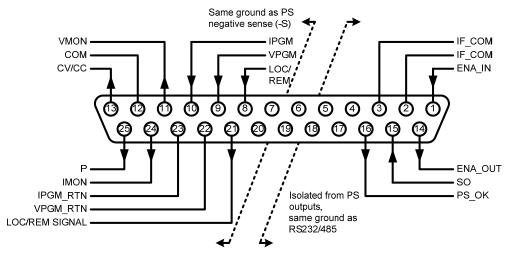
Fig.4-4: J1 connector terminals and functions
