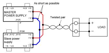
Fig.4-4: Parallel connection with local sensing
