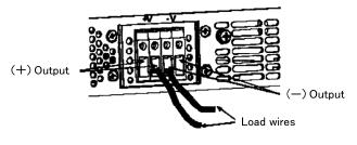
Fig.2-6: Load wires connection to the output terminal
