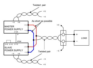
Fig.4-5: Parallel operation with Remote sensing
