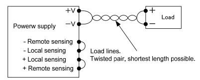
Fig.2-9: Single load connection, local sensing
