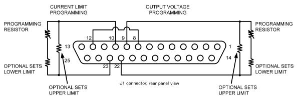
Fig.5-2: Remote resistive programming
