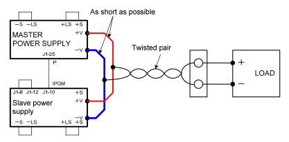
Fig.4-4: Parallel connection with local sensing
