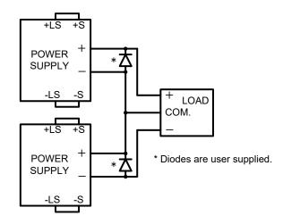
Fig.4-3: Series connection for positive/negative output voltages
