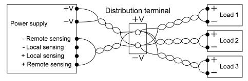
Fig.2-10: Multiple loads connection with distribution terminal
