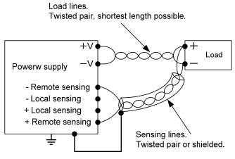
Fig.2-8: Remote sensing, single load
