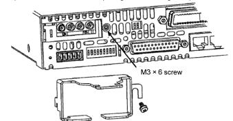
Fig.2-5: Shield assembly
