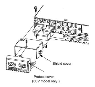
Fig. 2-3: Bus-bars shield mounting
