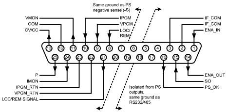
Fig.3-4: J1 connector terminals and functions
