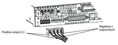
Fig.2-4: Load wires connection to the output connector
