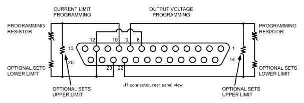
Fig.5-2: Remote resistive programming
