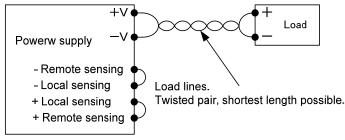
Fig.2-7: Single load connection, local sensing
