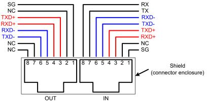
Fig.6-1: J3 rear panel IN/OUT connectors pinout
