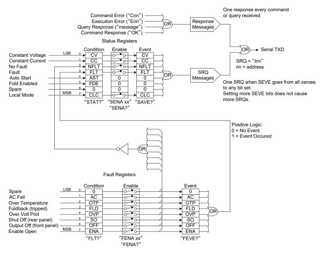
Fig.6-7: Status and Error Registers Diagram
