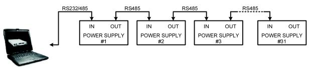
Fig.6-5: Multi power supplies RS232/485 connection
