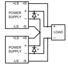
Fig.4-1: Series connection, local sensing
