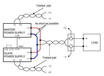
Fig.4-5: Parallel operation with Remote sensing
