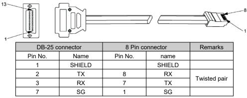
Fig.6-2: RS232 cable with DB25 connector
