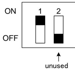
Fig 1-2: GP-IB select switch
